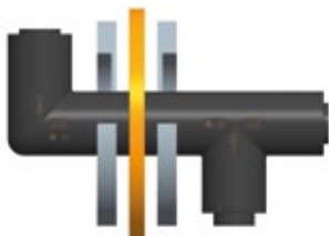
4. Warm up the welding areas
