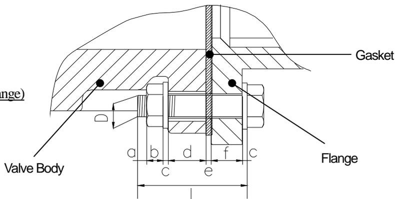
$$\text{Bolt Length [L]} = \text{Three threads beyond Nut of Bolt [a]} + \text{Thickness of Nut [b]} + \text{Thickness of Washer} \times 2 [\text{c}] + \text{Body [d]} + \text{Thickness of Gasket [e]} + \text{Thickness of Flange [f]}$$
