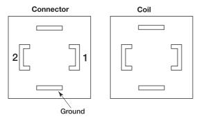
Terminals 1 & 2 are not polarity sensitive. Connector can be placed, wire facing up or down.
