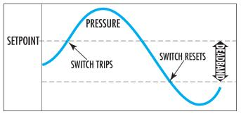
Deadband helps to prevent oscillation or "hunting". In other words, without sufficient deadband, the switch will be actuating and de-actuating too often. For applications where it is critical to de-actuate with less deadband, a 3 Amp switch is available. See specifications below.
