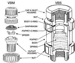
Series VB, not shown, has no SPIDER or NUT, and six (6) screws and nuts are used for assembly.
